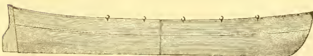
Fig. 9.—Elevation of Fore and Aft Sections, as a Cutter 25 feet long, and 8 feet beam, for ordinary ship's use.
